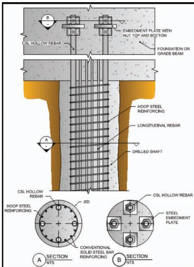
[FIG. 7] Typical CSL Hollow Threaded Rebar Detail
