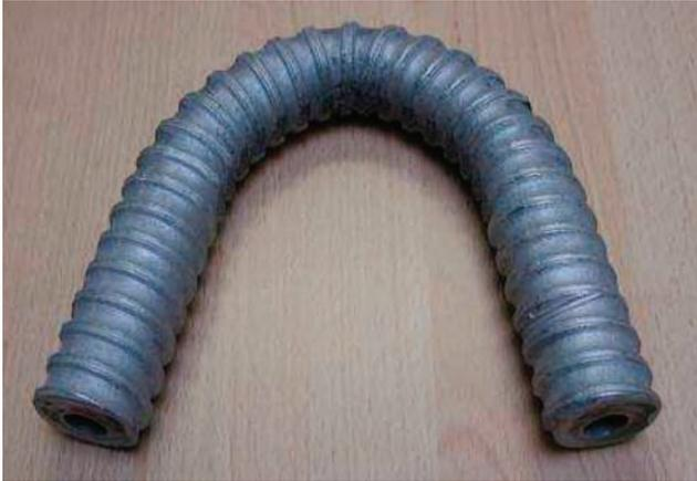
[FIG. 6] 180° bend test on Hollow Threaded Rebar
