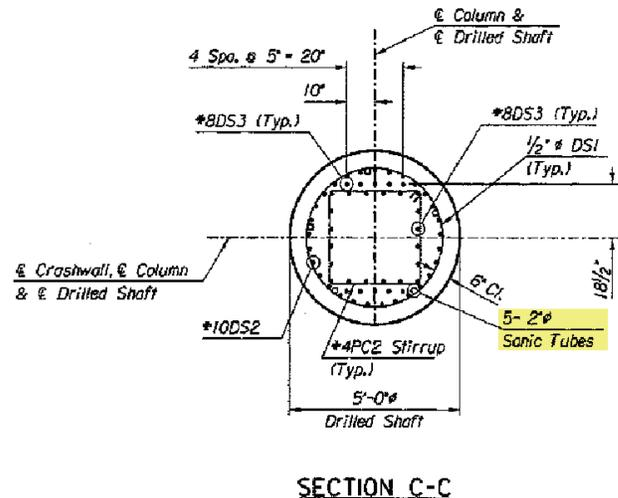
[Fig. 4] Example of Drilled Shaft with 5 each 2" sonic tubes. Sample taken from Kansas Department of Transportation
